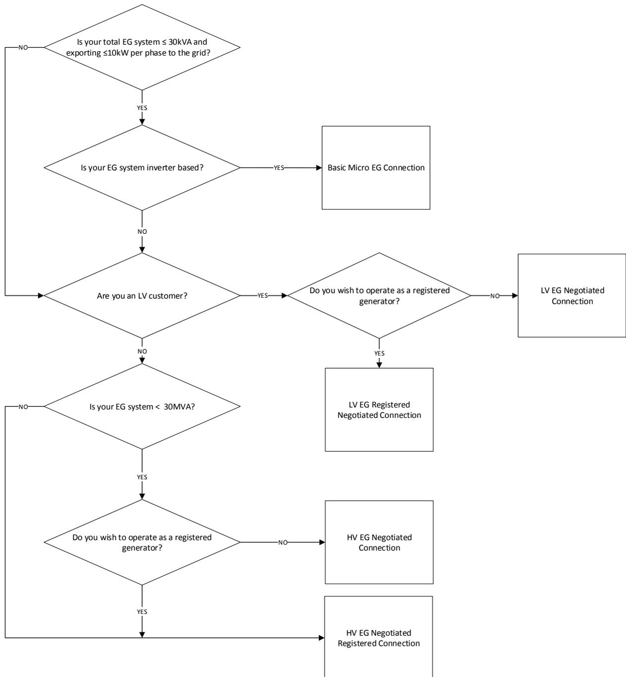
Figure 2 Type of EG Connections
